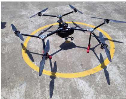
Fig. 12 Hex-Copter for Electro Magnetic Survey.
