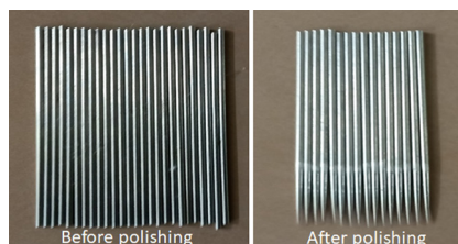
Fig. 24 Medical grade SS surgical needles before and after electropolishing.
