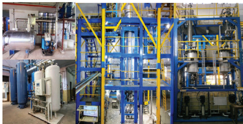
Oxygen-enriched air blown pressurized fluidized bed refractory lined gasifier at CSIR-CIMFR
