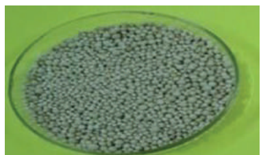
Specialty Borosilicate Glass Bead for Nuclear Waste Immobilization
