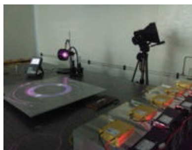
Test bed system for generating 500W CW power lasers
