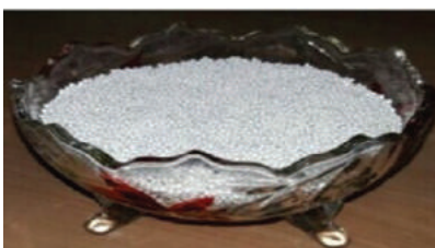
Specialty Borosilicate Glass Bead for Nuclear Waste Immobilization
