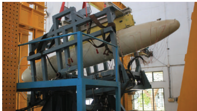
Test set-up for LCA fuel drop tank under slosh and vibration loading
