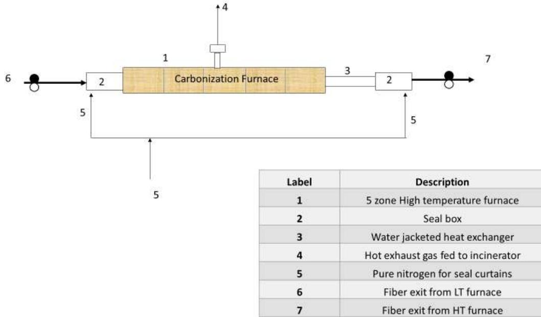
Fig.6 Schematic representation of the carbonization furnace
