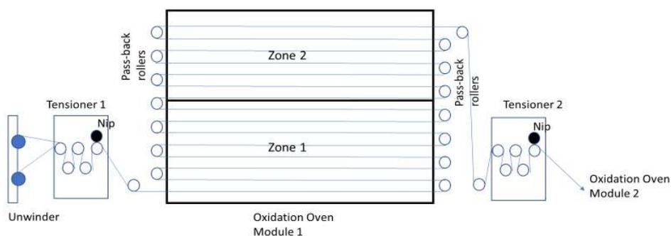
**Fig.3 Representation of Stabilization Oven module 1**
