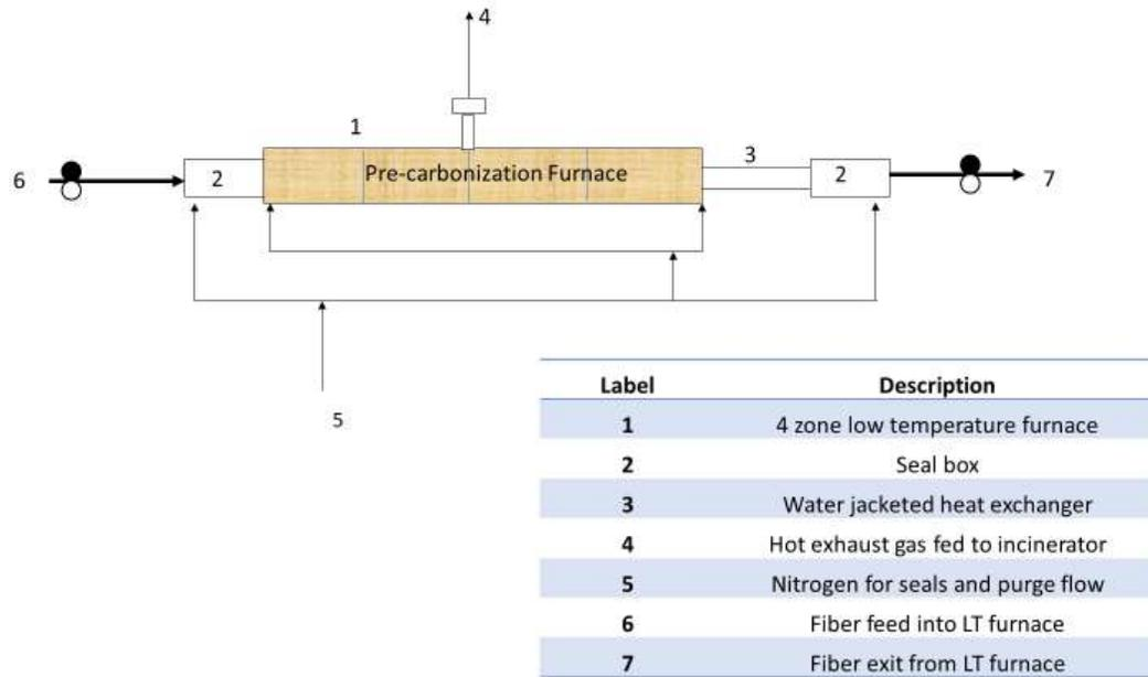
Fig.5 Schematic representation of Pre-carbonization furnace
