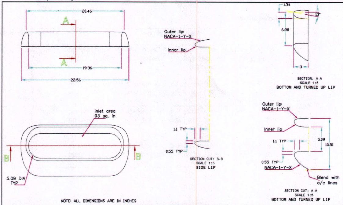
Figure 2: Saras Mk II Aircraft - Engine Air Intake Lip
