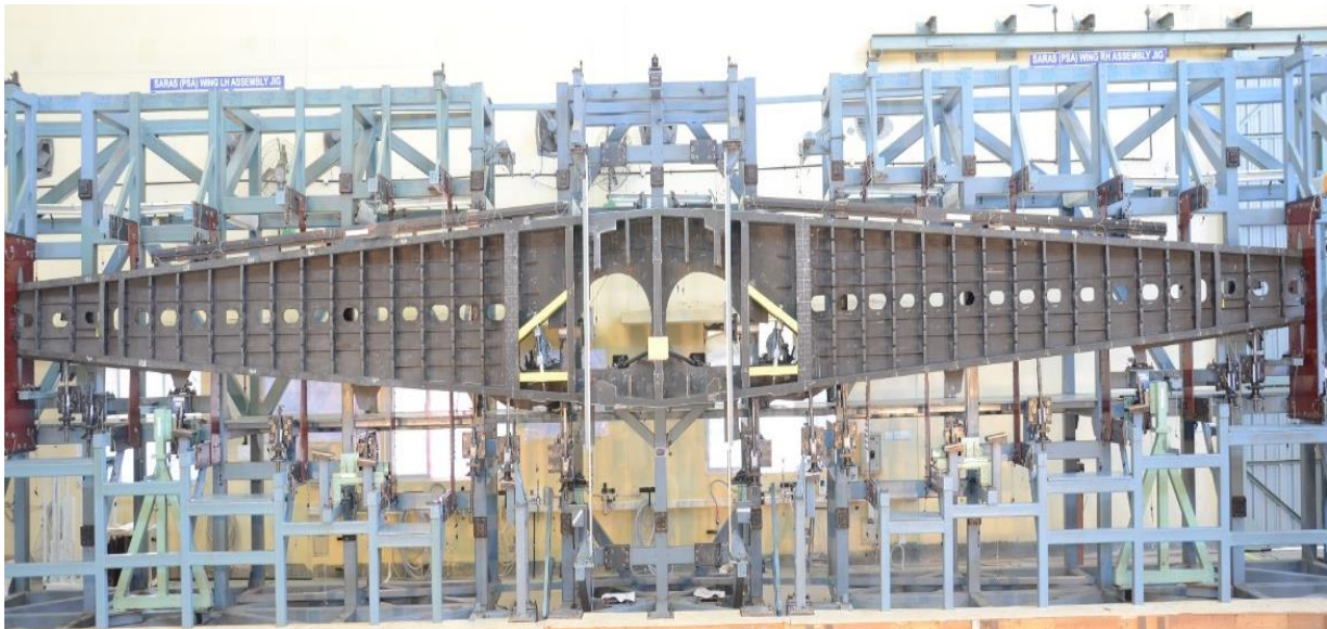
Fig. 17: Typical representation of wing assembly Jig
