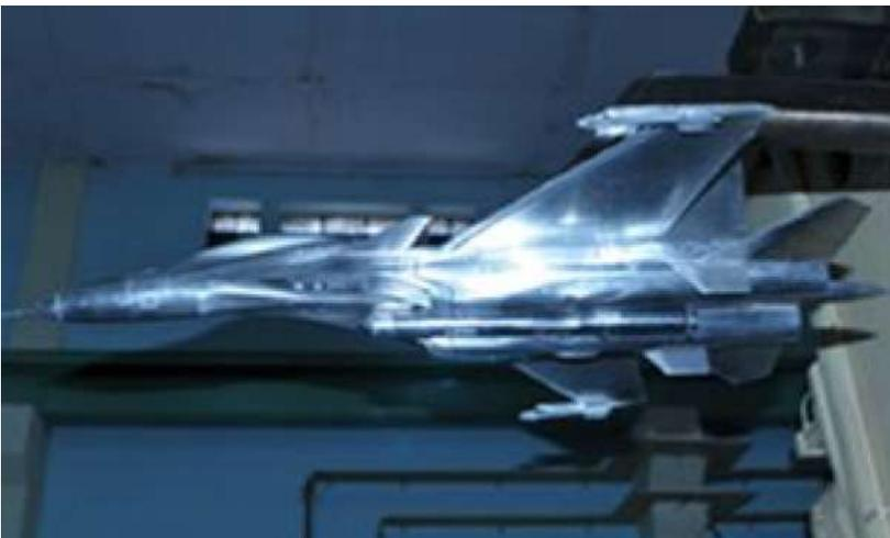
A Su-30 MKI model, the largest aircraft model, was designed, fabricated and commissioned at a record time at NAL's National Trisonic Aerodynamic Facilities (NTAF). [A trisonic wind tunnel is capable of testing flight vehicles at subsonic, transonic and supersonic speed ranges].
